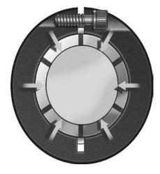
The D-LOK concentric clamp collar, with a single standard hex head cap screw and relief slot, provides greater holding power over competitive products. The collar, installed over the slotted inner ring, locks the bearing on the shaft concentrically without marring or burring and provides a 360° clamping force to the shaft with minimal run out (T.I.R.) for less vibration.
