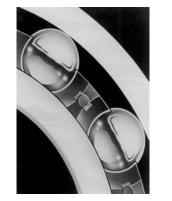
Ball cage is made of heat-stabilized nylon, reinforced with 33% short strand fiberglass. This non-metallic container operates in higher temperatures with less water absorption and retains natural lubricity and flexibility.
